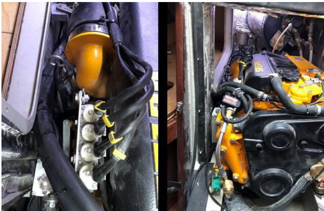
Fig 9. DME/mixed fuels injection system and the modification of Photon engine
