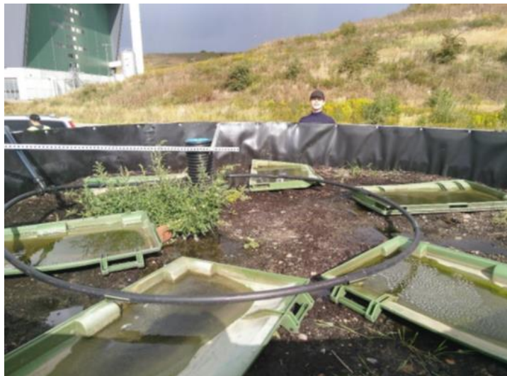
Figure 14 Improvement of the water dispersing system in the hybride filter
