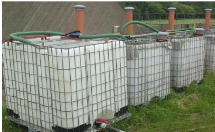
Figure 6 Air purification system formed by 1 m3 IPC container with bark filter.
